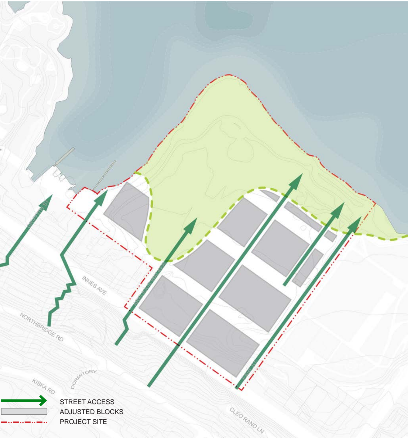
The long, rectangular block pattern would block movement, so large blocks will be broken down into smaller, more compact blocks. Smaller blocks promote walkability and waterfront access.
