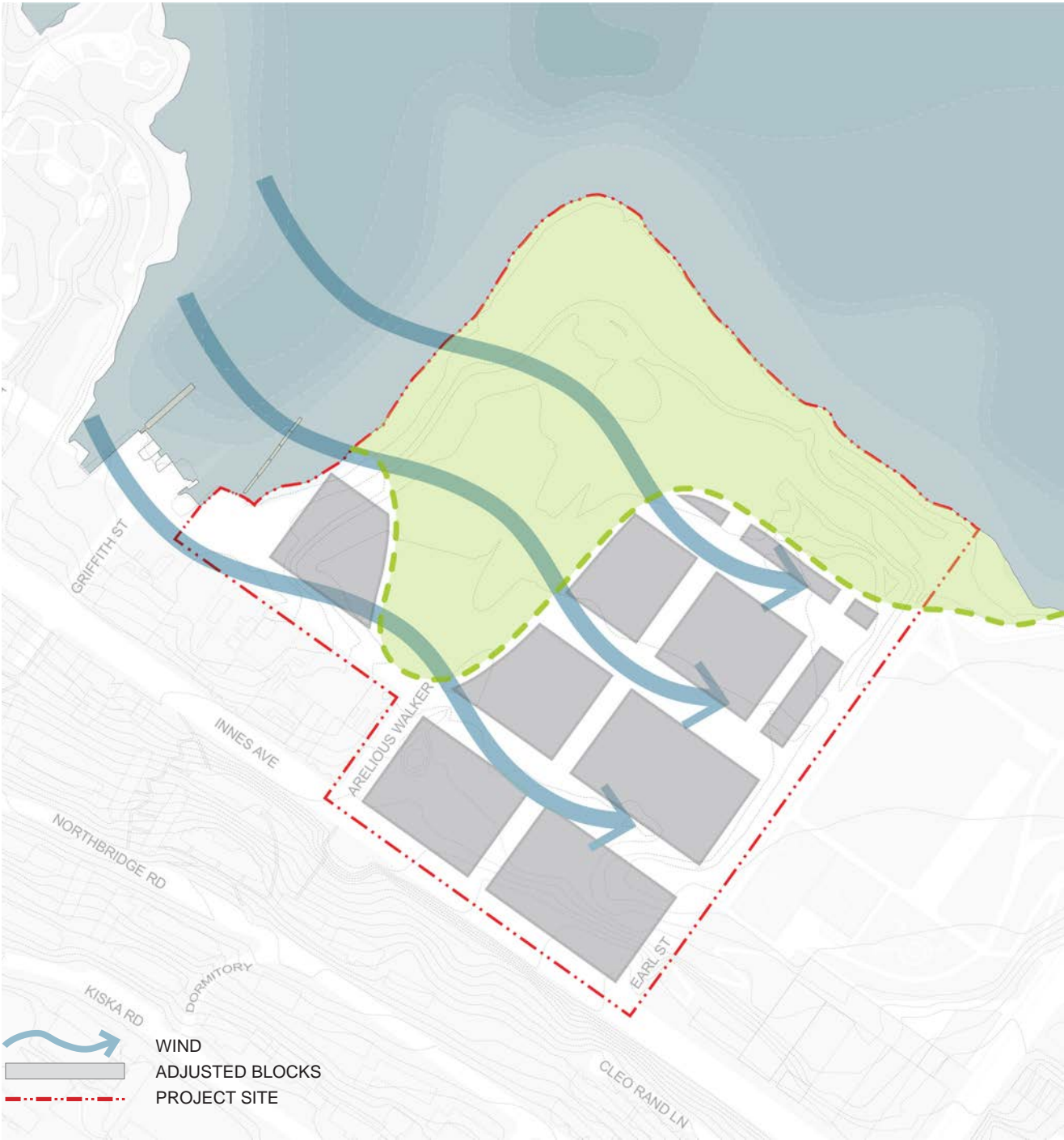
The Project Site has its own microclimate with prevailing wind originating from the northwest. The existing city grid has a similar orientation and the combination of these two factors would result in uncomfortable wind effects along the long faces of the city blocks. The current block orientation would channel winds into streets and public space.
