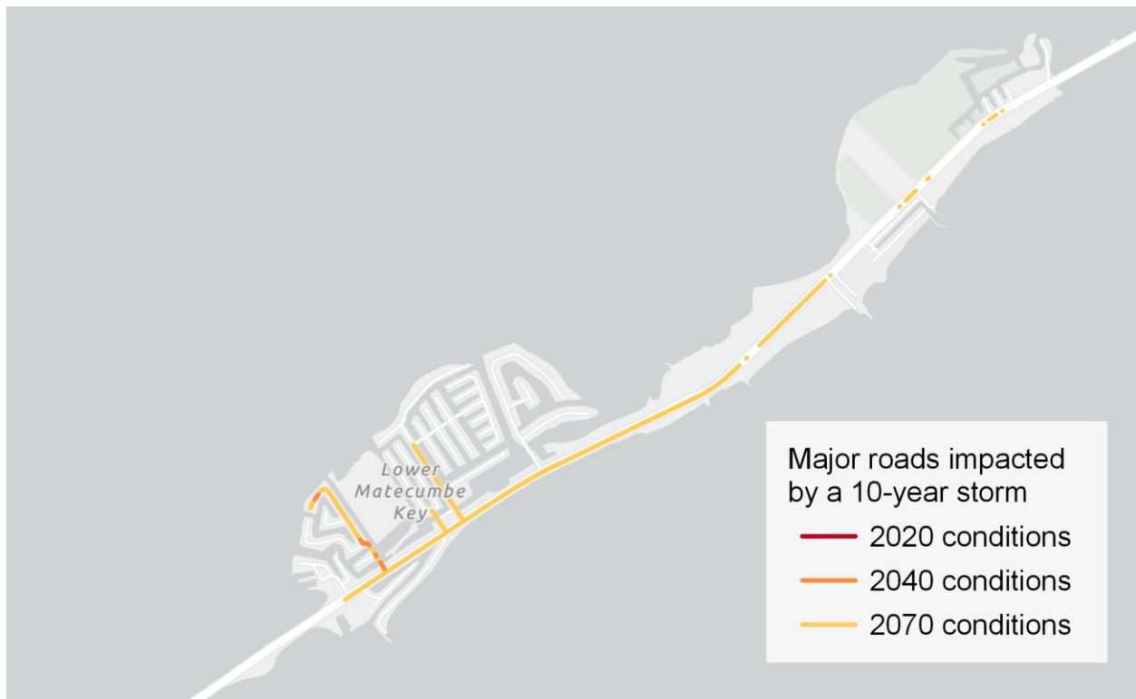
Figure 10: Major roads impacted by the 10-year storm by horizon year on Lower Matecumbe Key
